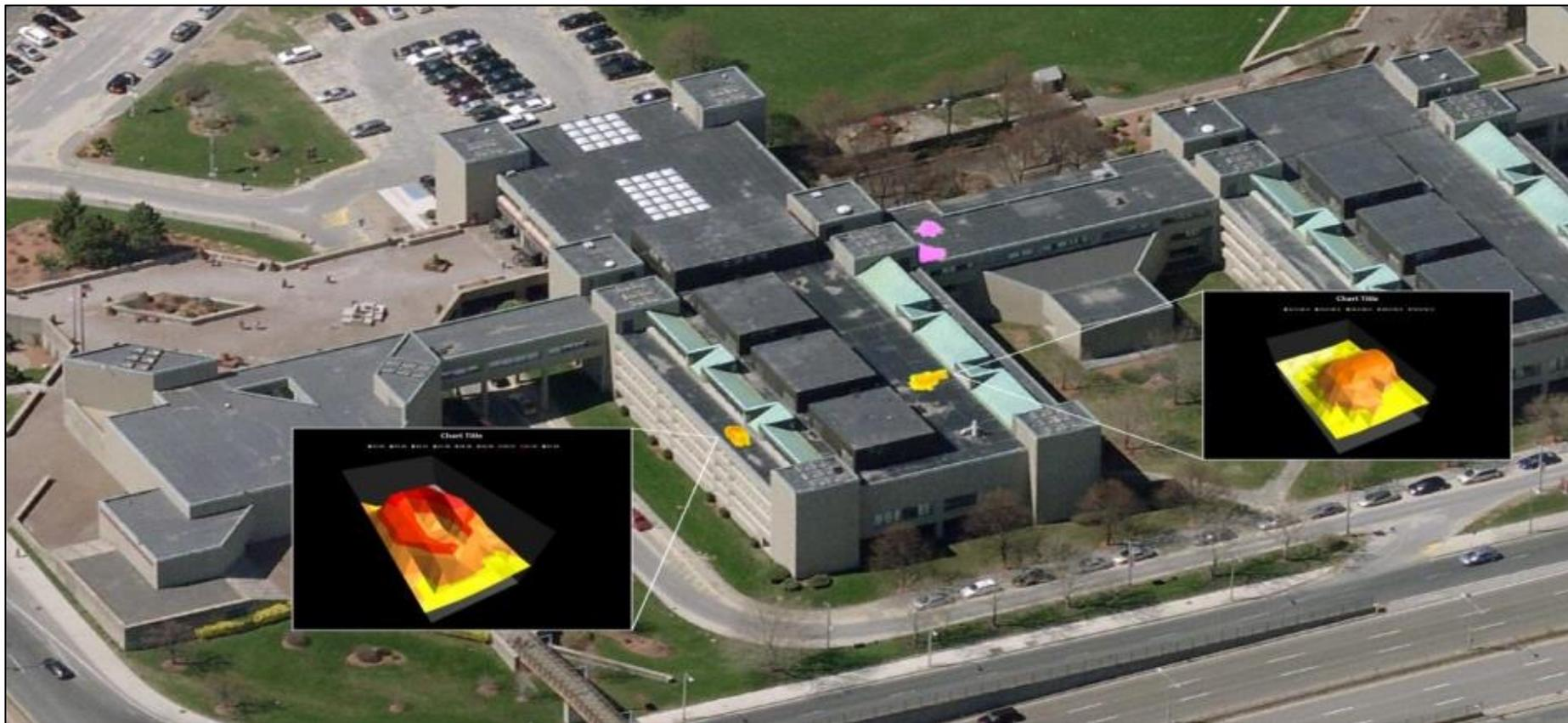
**Energy Calcs derived From Thermal Patterns of Moisture Damage**
